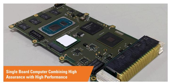
General Dynamics has developed the Single Board Computer (SBC) to provide a high performance 3U VPX module that can be used in systems that require high assurance levels. The processor can be used single-core or multicore to provide improved performance and has built-in General Purpose Graphics Processing Unit (GPGPU) for high resolution display graphics and parallel compute.
